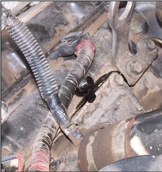
Fig. 4 – Passenger Side HPX Fitting Installed
