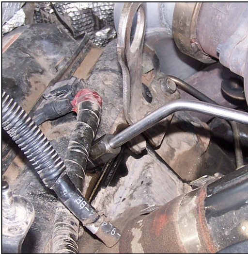
Fig. 6 – Passenger Side HPX Tube Installed
