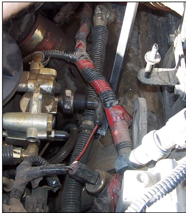
Fig. 3 - Using a Pry Bar to Bend Hose Clamp
